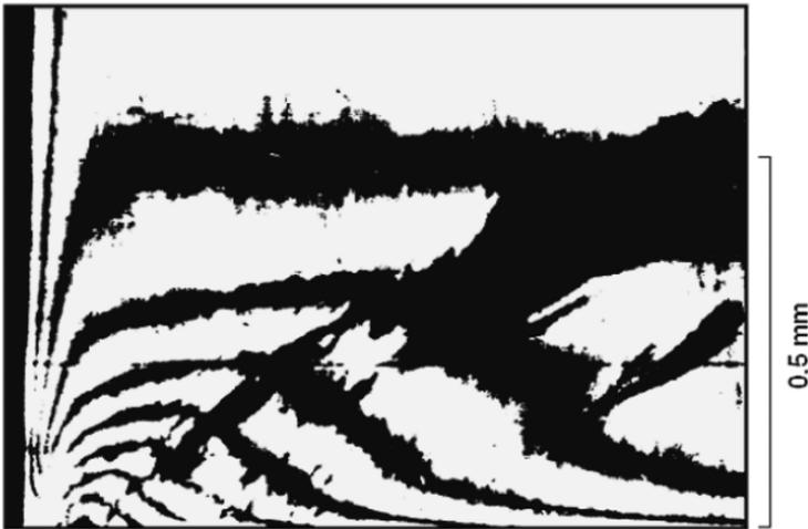
**Fig. 1.10.** A fragment of chronographic scanning of the optical image near the cathode. Tracks show moving bubbles. Bands whose shapes are close to voltage pulse waveforms show the Kerr bands. Bending of these bands shows the motion of injected charges
