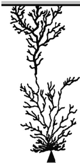
**Fig. 4.17.** Schematic image of the discharge in transformer oil propagating over the pressboard surface [52]
